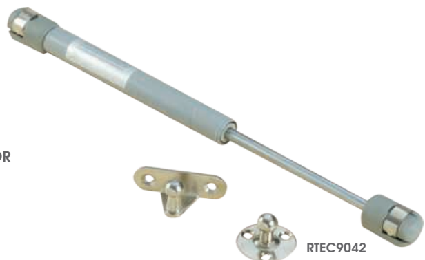
RTEC9042 GAS LIFT 270MM 200N Load Capacity 4.5kg N110 Extended length 243mm Includes 2 Snap-on ball fittings for solid and MDF doors
