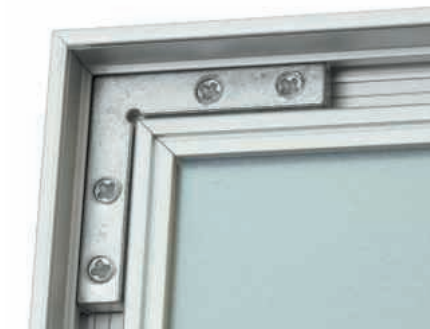
RFCA4 CORNER CONNECTOR 4 Connectors required per door 4 Fastening screws Minimum starting point for hinge is 78mm from middle line of corner connector.
